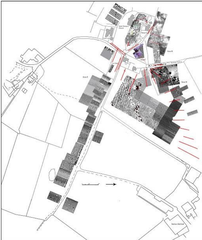
Figure 1: Plan of Mellor hilltop indicating the areas covered by the various different types of geophysics and the results. The red coloured lines represent coverage by Ground Penetrating Radar (GPR).
